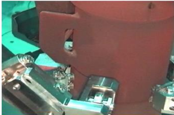
Cut through a jet pump using a band saw
